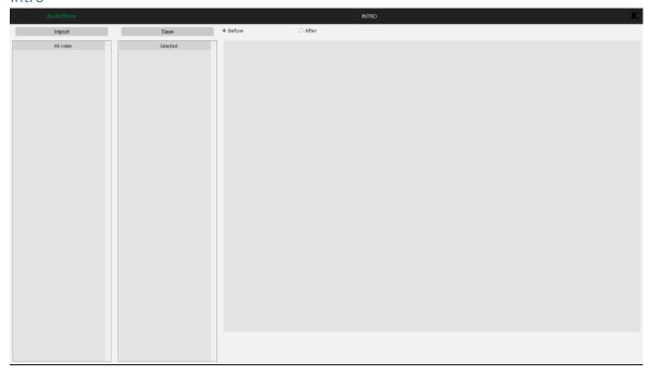
In this window it is possible to import video files in mp4 format. The video that will be used in the preset as a intro is dragged with the mouse into the "Selected" column. After selecting, you must click "Save".
